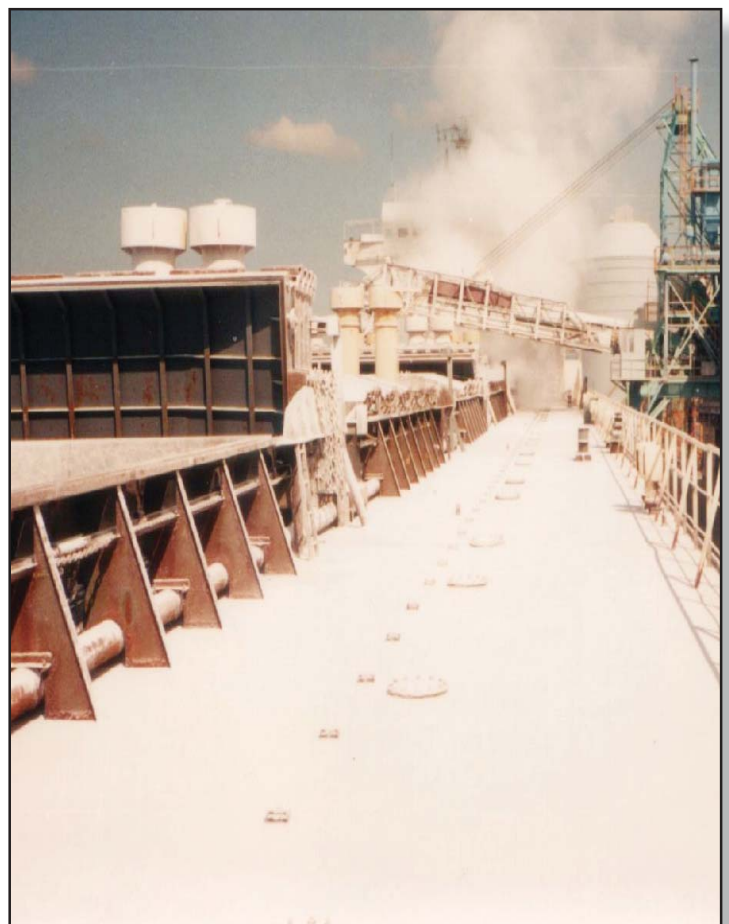
Example of nuisance dust during discharge as evidenced by dust cloud and errant material build-up on deck and ship's gear.
